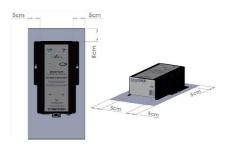
The unit can be wall mounted in a vertical orientation only with the connections at the bottom.
