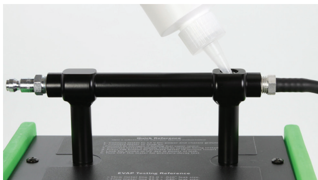
Fig. 5: Filling the UltraTraceUV® smoke solution
