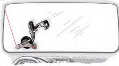
Upon reaching the top right corner, change the position again to the top left corner (Fig. 5). Then change position to the bottom left corner (Fig. 6) and complete the removal process.
