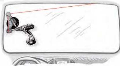
Use the cordless screw driver slowly to the right, adjusting the speed depending on load. During this process hold the removal protector internally between the windscreens removal cord and the dashboard, shaft or roof lining, so that the interior of the vehicle cannot be damaged. Now continue with the removal process until the windscreens removal cord has reached the bottom right corner .
