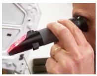
The instrument also features an eye guard to prevent stray light from entering the eyepiece and causing reflections.
