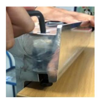
Position the hoist pad with retaining feet facing down on a work bench or table top in such a way that the pad is supported against the edge of the table. The retaining feet should rest in the groove and must not twist or turn. Loosen the bolt and unscrew. Unscrewing can be somewhat tricky as the caulking of the first threads has to be overcome. Hoist pads and springs are to be re-used.
