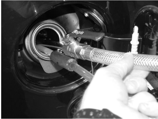
Suction handle & fume recovery tube in fuel filler tube on vehicle.
