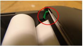
If the switch is in the incorrect possition, put a little screwdriver between the top of the switch and the bottom of the housing. Push the switch on the top to flip it.
