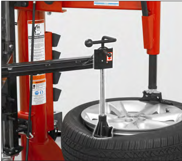
Press arm pushes tire into drop center for mounting and demounting operations
