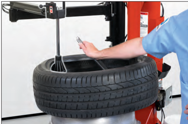
Lifting hook aids the demounting of heavy tires.
