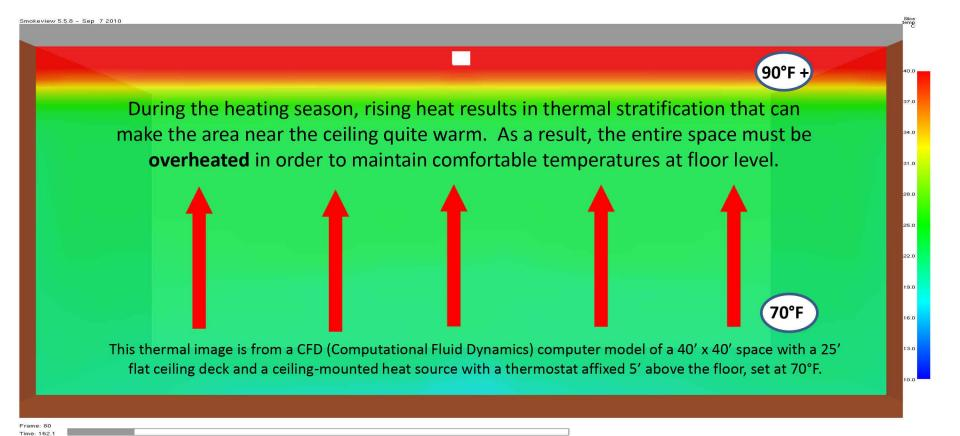
The difference in temperature between the floor and the ceiling can be significant: 0.5°F to 1°F per foot, or more, above 5 feet. For example, during the heating season, a space with a 30' ceiling could have a temperature differential between the floor and ceiling of 12.5°F to 25°F, depending on variables such as outside temperature and building insulation.
