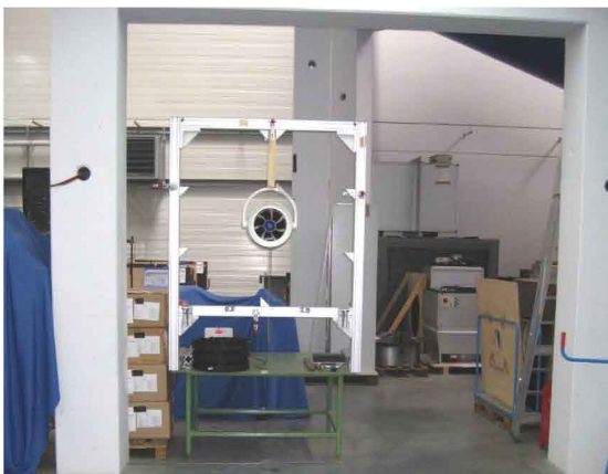
Set-up of throwing range measurements of FN025-4ED.W8.A7
