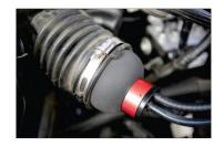
Ideal for sealing any large and/or irregular shaped opening such as those now common to induction systems and exhaust systems.
