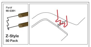
The **Z-Style** staples are great for exceptionally strong plastic repair, made for stitching broken seams and cracks.
