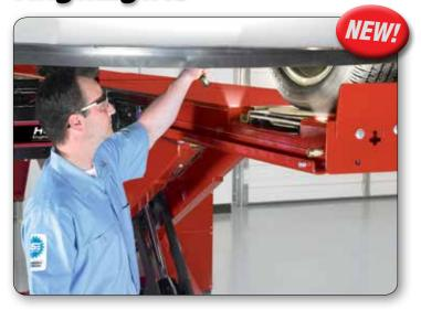
AlignLights is available for most Hunter alignment lifts as an installed option or can be retrofitted to many previously installed lifts.
